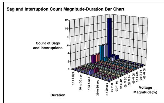
Figure 2d: Voltage Sag Statistical Analysis
