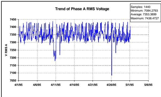
Figure 2a: Trend of Steady-State Sampled Data
