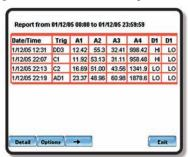
systems. If desired, records of data values as they existed just prior to a triggering event can be included in the stored data file. The touch of a button will display a scrollable spreadsheet report of all currently logged data, including time and event indication.
