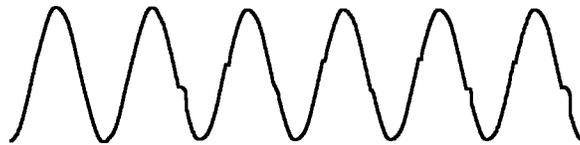
**Figure 2.** Waveshape with notching caused by a loose connection.
