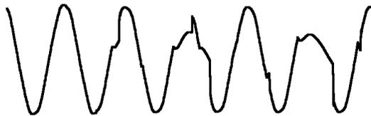
**Figure 3.** Waveshape as loose connection progressed.
