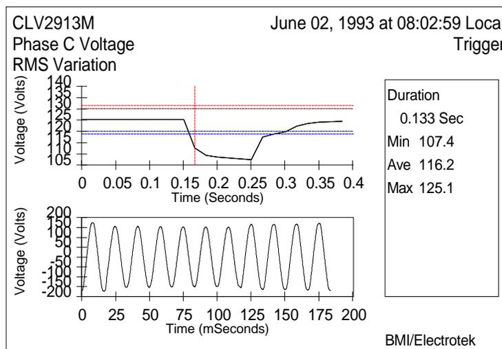
**Figure 9.** Example voltage sag event with a magnitude of 107V and a duration of 0.133 second.
