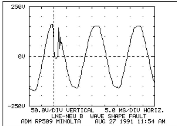
**Figure 8.** Wavelshape fault during the operation of a voltage regulator.
