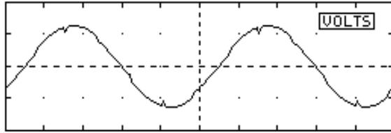
**Figure 1.** Example of voltage notching due to power electronic devices.
