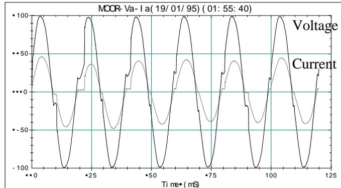
**Figure 4.** Voltage and current waveshapes from circuit with a loose connection.
